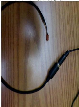
Plug the clock power adapter into the Brick Power Adapter
